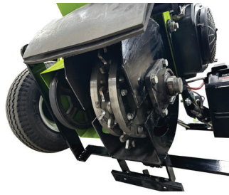
Easy to Access Drum to Rearrange or Replace Bits
