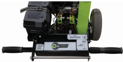
Belly Bar Disengages Clutch Allowing Drum Assembly to Stop but Does Not Kill the Engine
