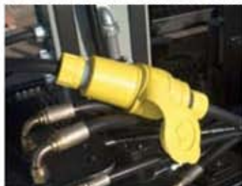
Plug connection for extension heat.
