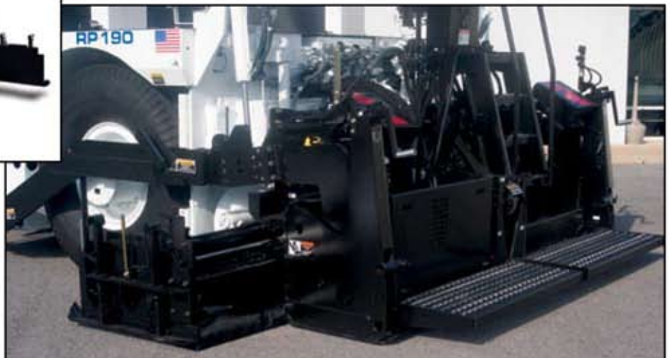
Top: Front view of SC screed with extension retracted. Right: Rear view of SC screed with extensions out.
